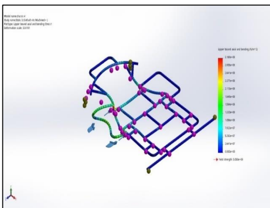
Figure 9: Side Impact on Aluminium Alloy Chassis With Factor of Safety = 1.6 and Maximum Displacement 15.828 mm
